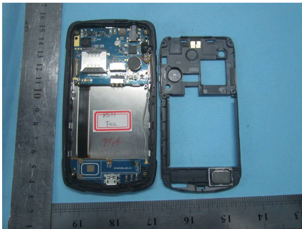
Cover Off Without Housing - Top View
