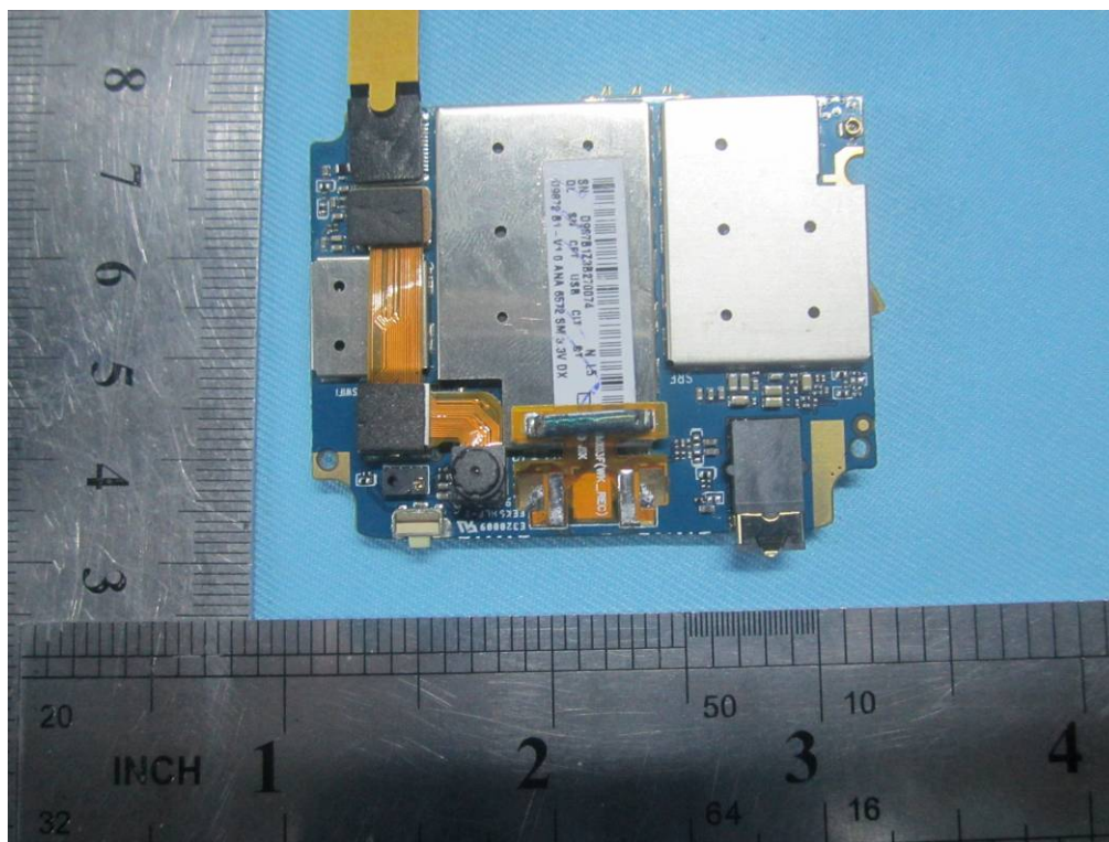
Mainboard With Shielding - Front View
