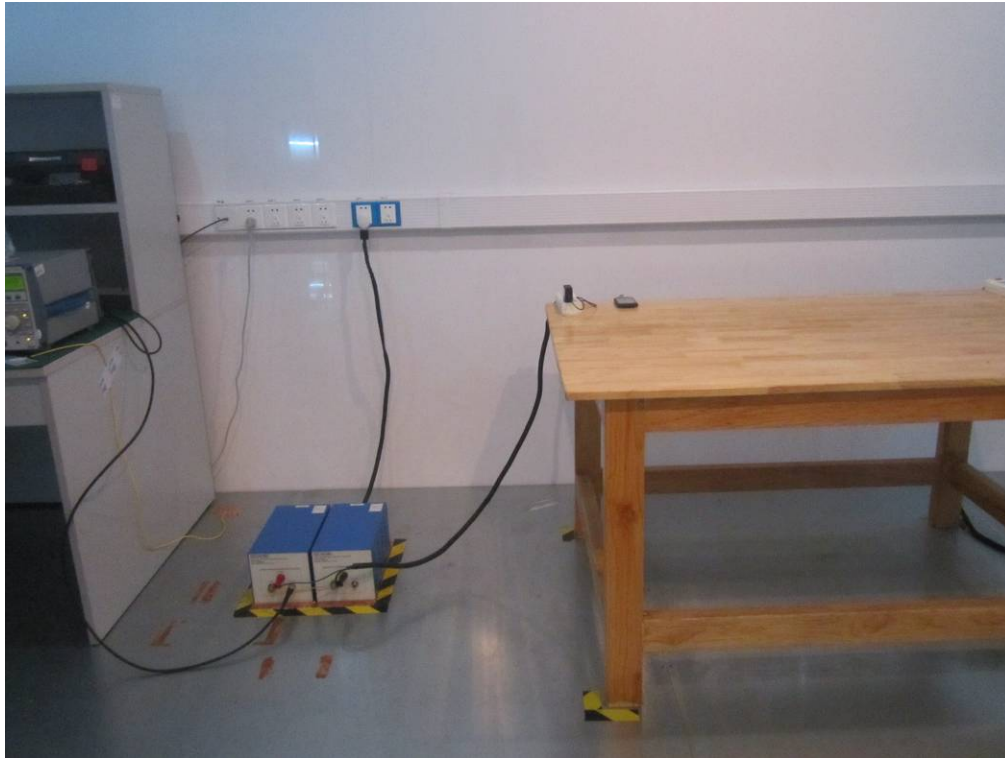
Conducted Emissions Test Setup Front View
