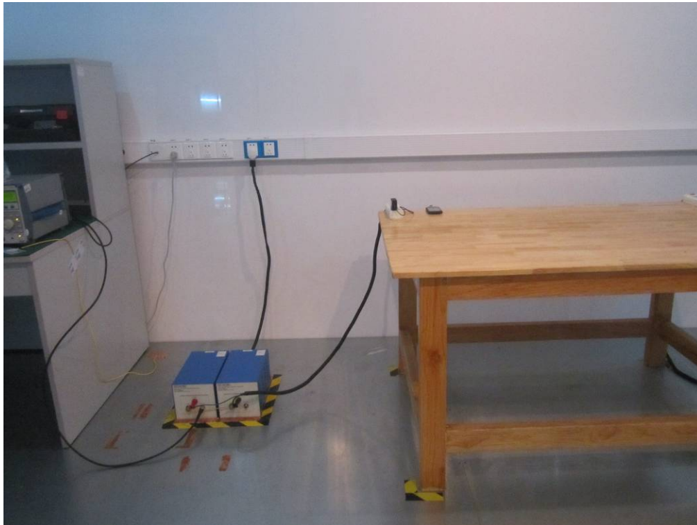
Conducted Emissions Test Setup Front View
