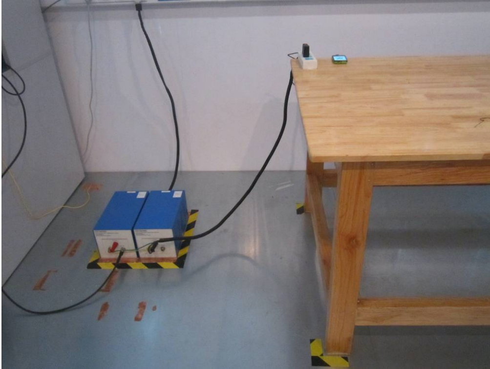
Conducted Emissions Test Setup Front View
