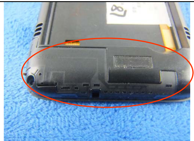
GSM/PCS/UMTS-FDD Antenna View
