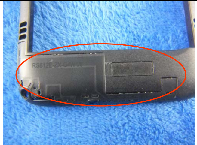
GSM/PCS/UMTS-FDD Antenna View
