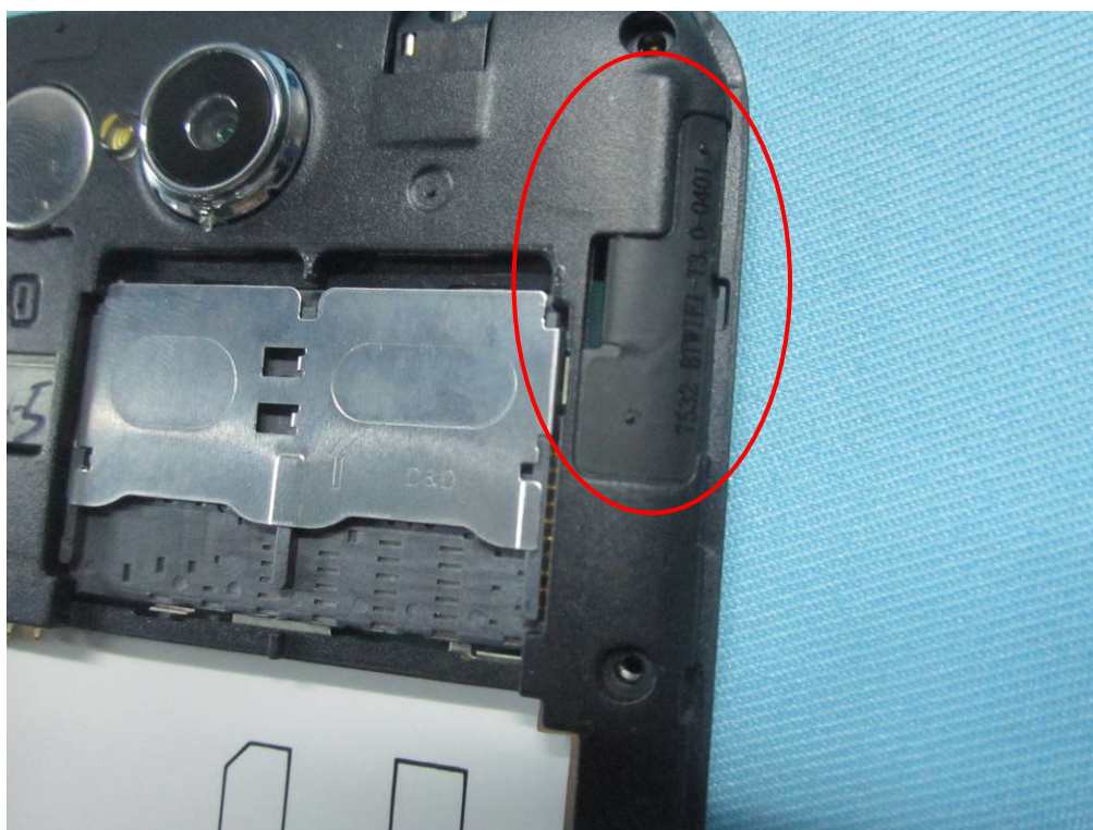
BT/WIFI Antenna View
