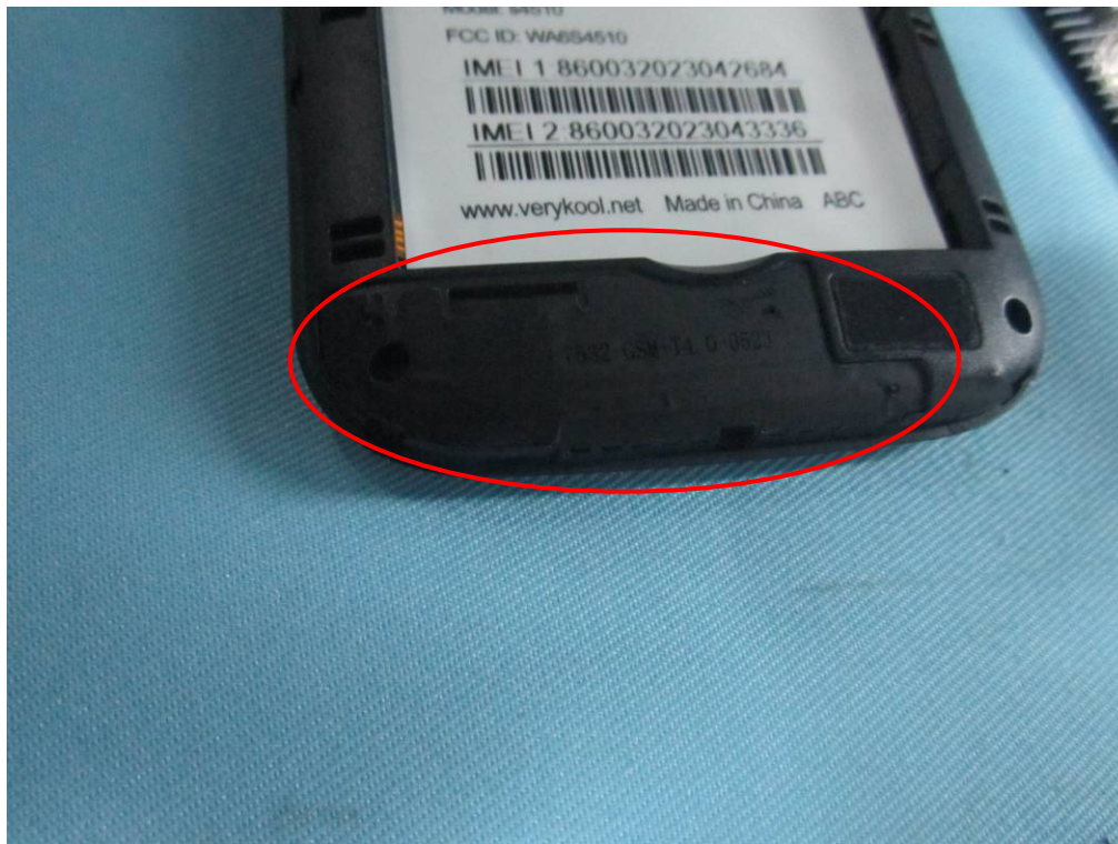
GSM/PCS/UMTS-FDD Antenna View
