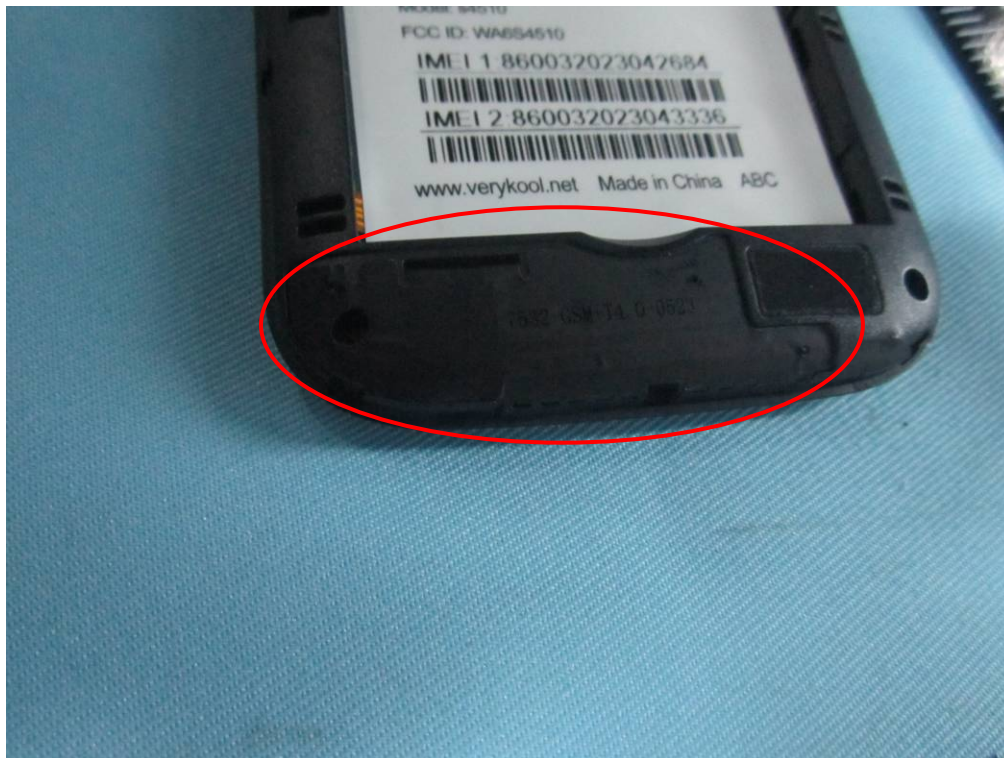
GSM/PCS/UMTS-FDD Antenna View
