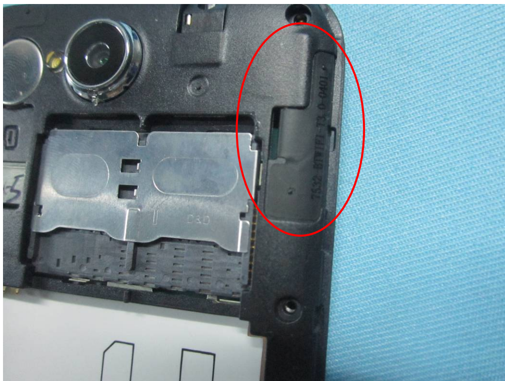
BT/WIFI Antenna View
