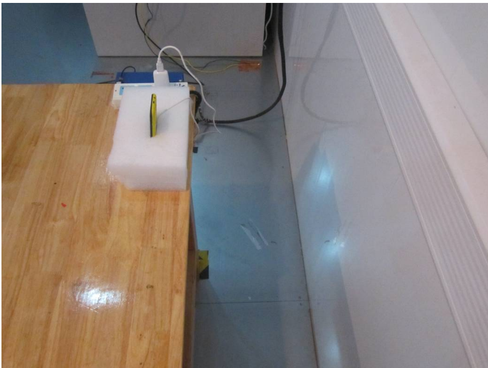
Conducted Emissions Test Setup Side View
