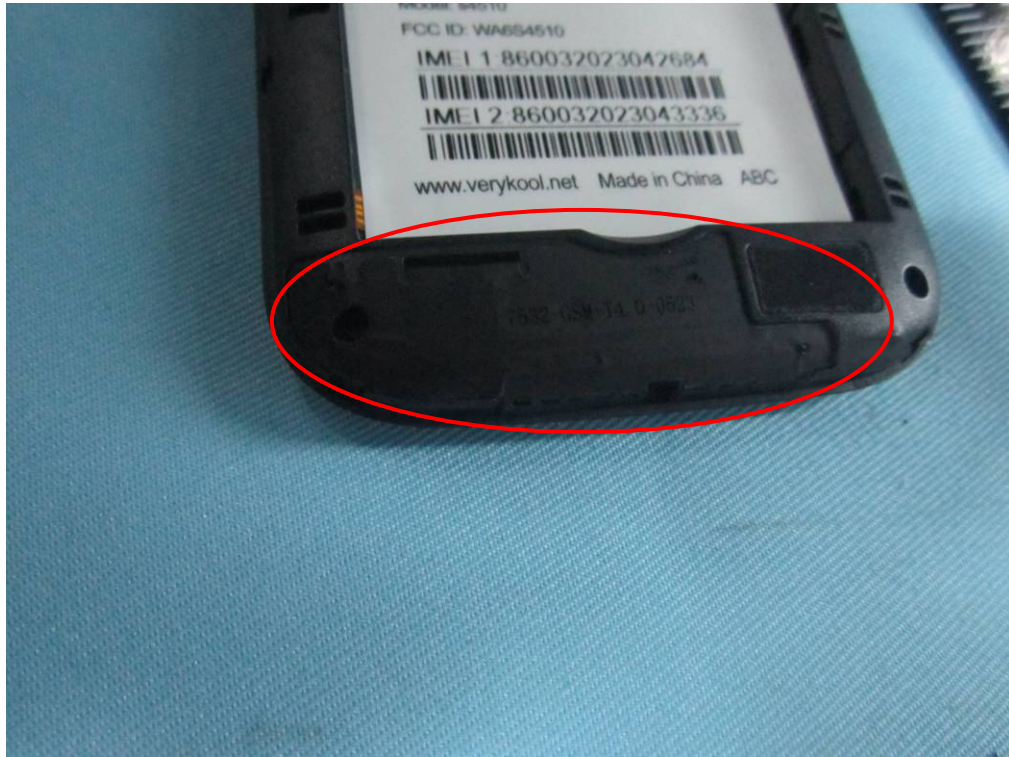
GSM/PCS/UMTS-FDD Antenna View
