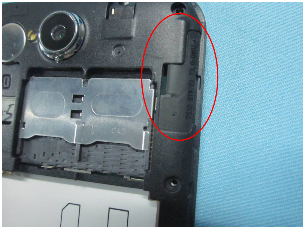
BT/WIFI Antenna View
