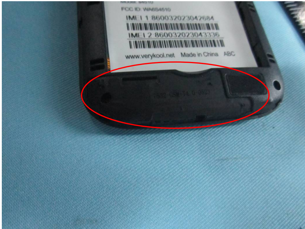
GSM/PCS/UMTS-FDD Antenna View
