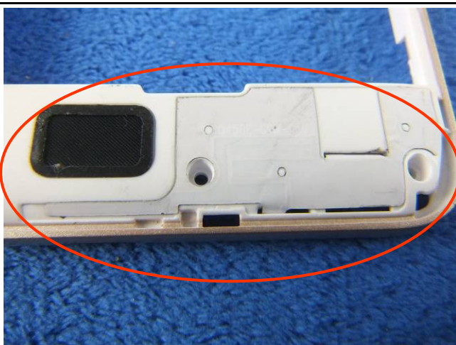
GSM/PCS/UMTS-FDD Antenna View
