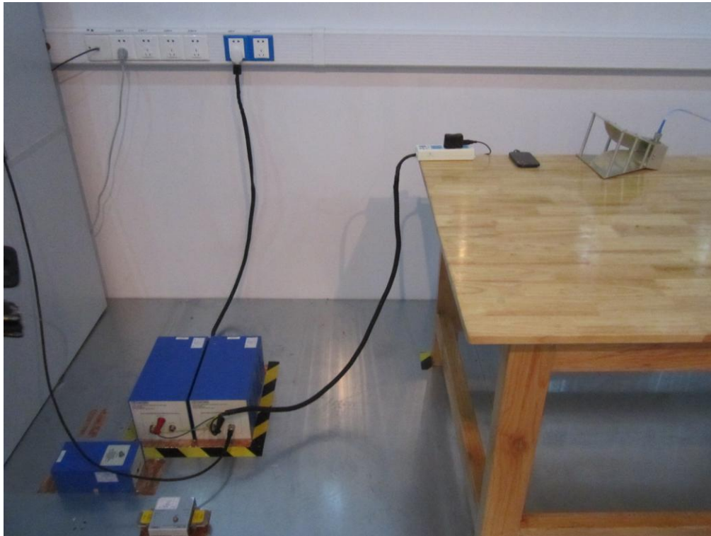
Conducted Emissions Test Setup Front View
