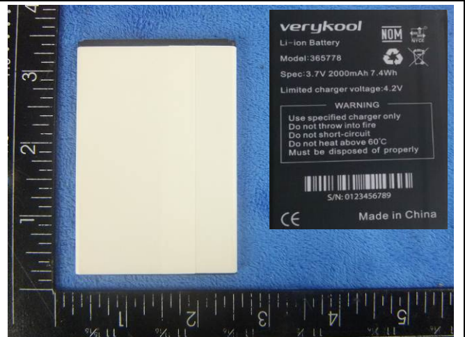
Battery Label - Rear View
