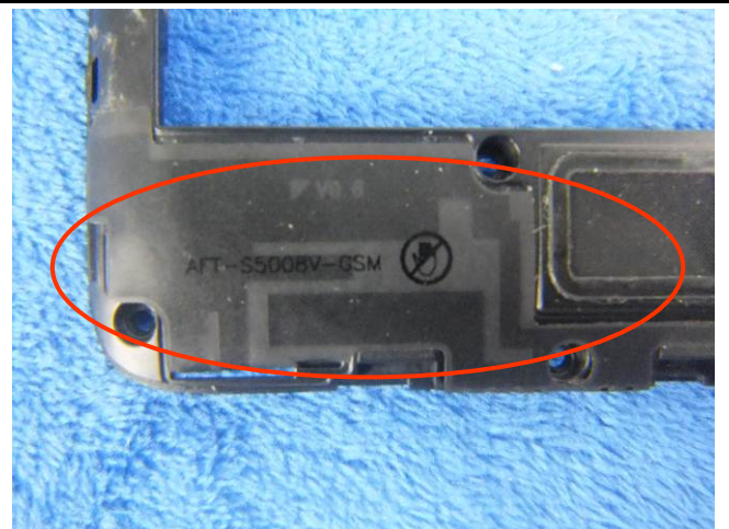
GSM/PCS/UMTS-FDD Antenna View
