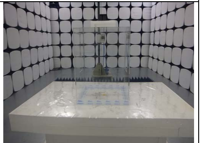
Radiated Spurious Emissions Test Setup Above 1GHz
