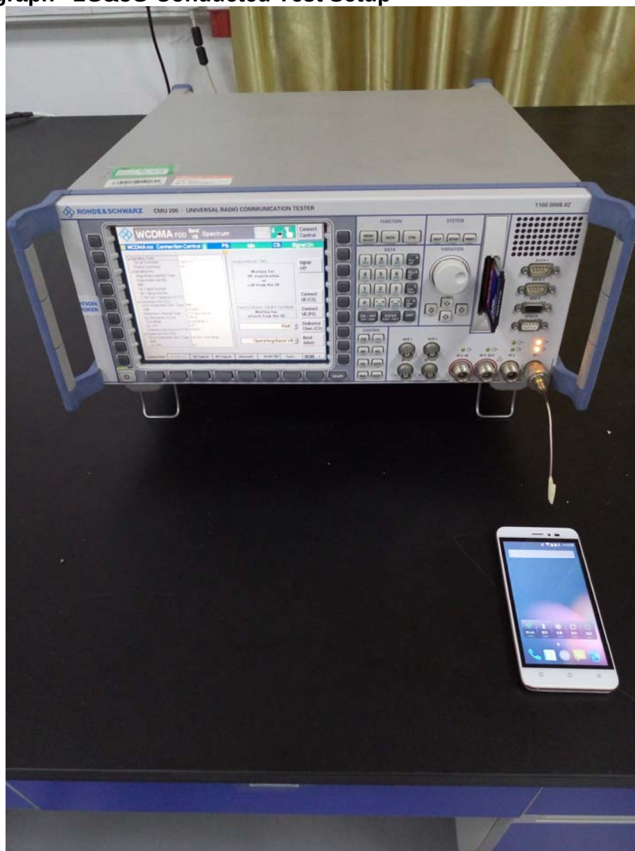
Photograph –2G&3G Conducted Test Setup
