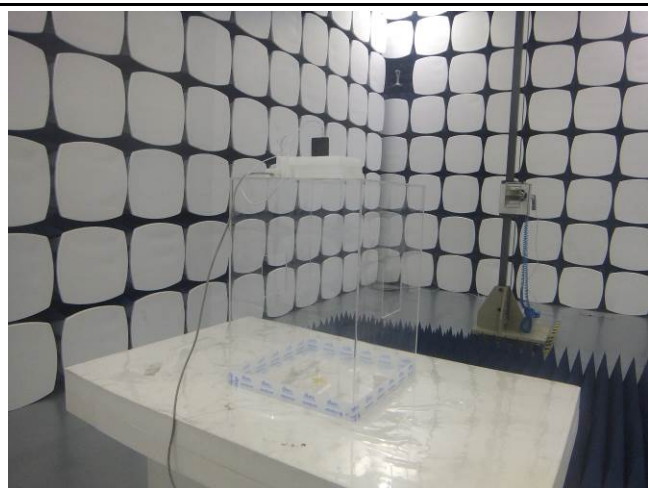
Radiated Spurious Emissions Test Setup Above 1GHz
