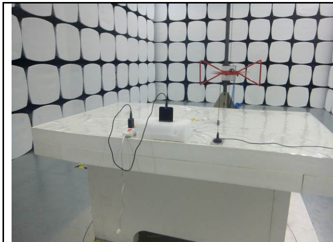
Radiated Spurious Emissions Test Setup Below 1GHz
