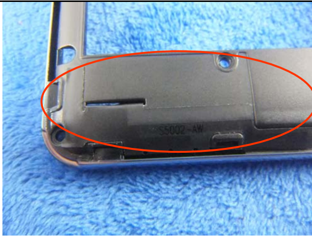
GSM/PCS/UMTS-FDD Antenna View
