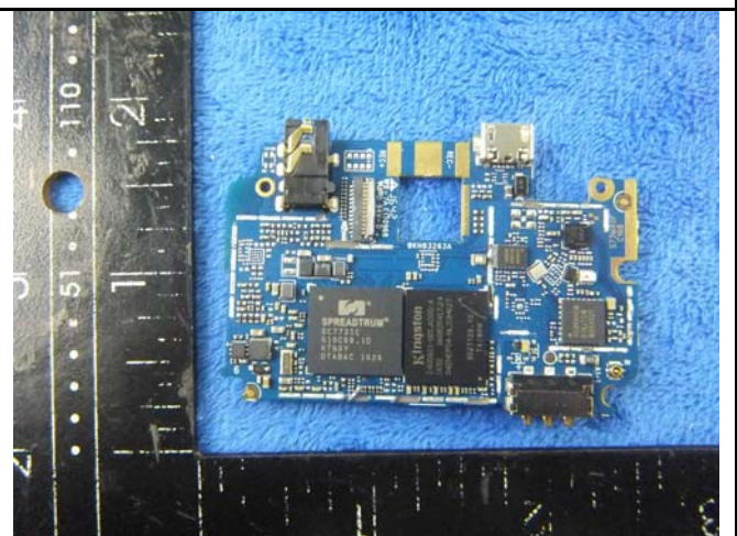
Mainboard without Shielding - Front View
