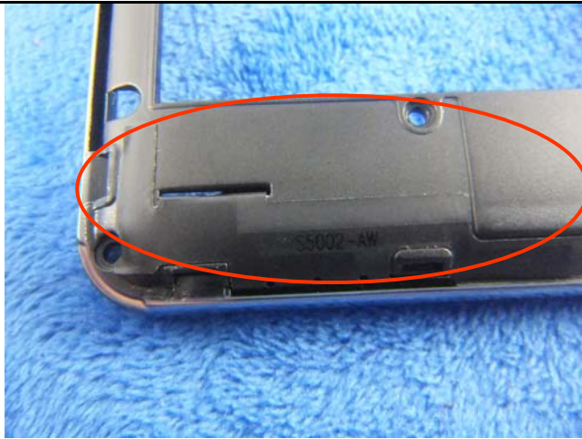
GSM/PCS/UMTS-FDD Antenna View
