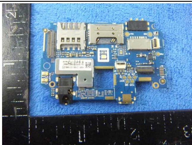
Mainboard with Shielding – Rear View
