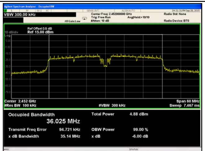
802.11n40 6dB Bandwidth - High CH 2452
