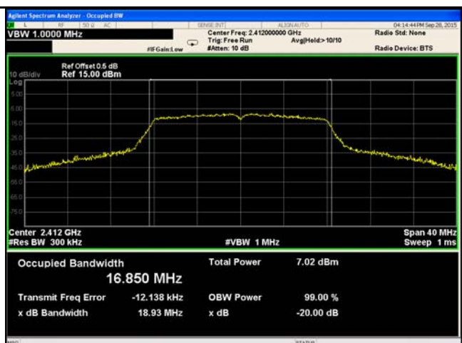
802.11g 20dB Bandwidth - Low CH 2412
