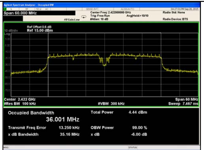
802.11n40 6dB Bandwidth - Low CH 2422
