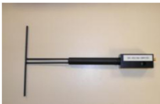
Figure 1 – Satimo COMOSAR Validation Dipole
