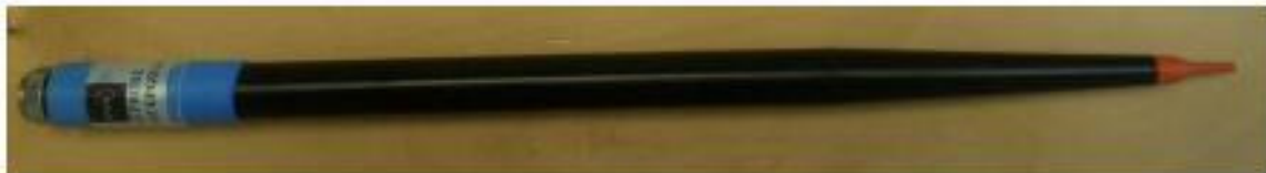
Figure 1 – MVG COMOSAR Dosimetric E field Dipole
