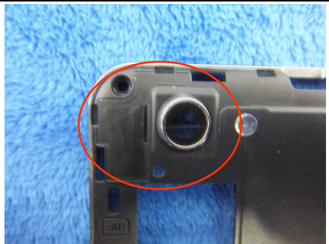
WIFI/BT/BLE/GPS - Antenna View
