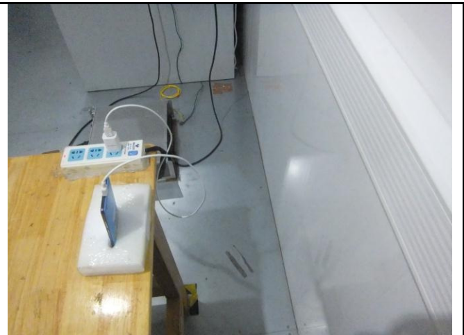
Conducted Emissions Test Setup Side View
