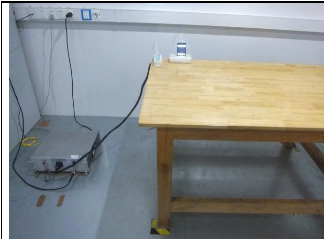
Conducted Emissions Test Setup Front View
