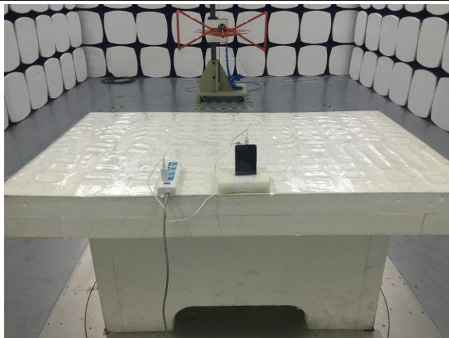
Conducted Emissions Test Setup Front View
