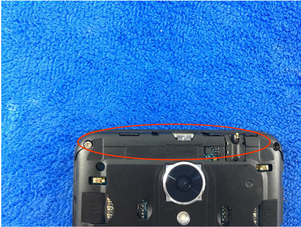
WIFI/BT/BLE/GPS - Antenna View
