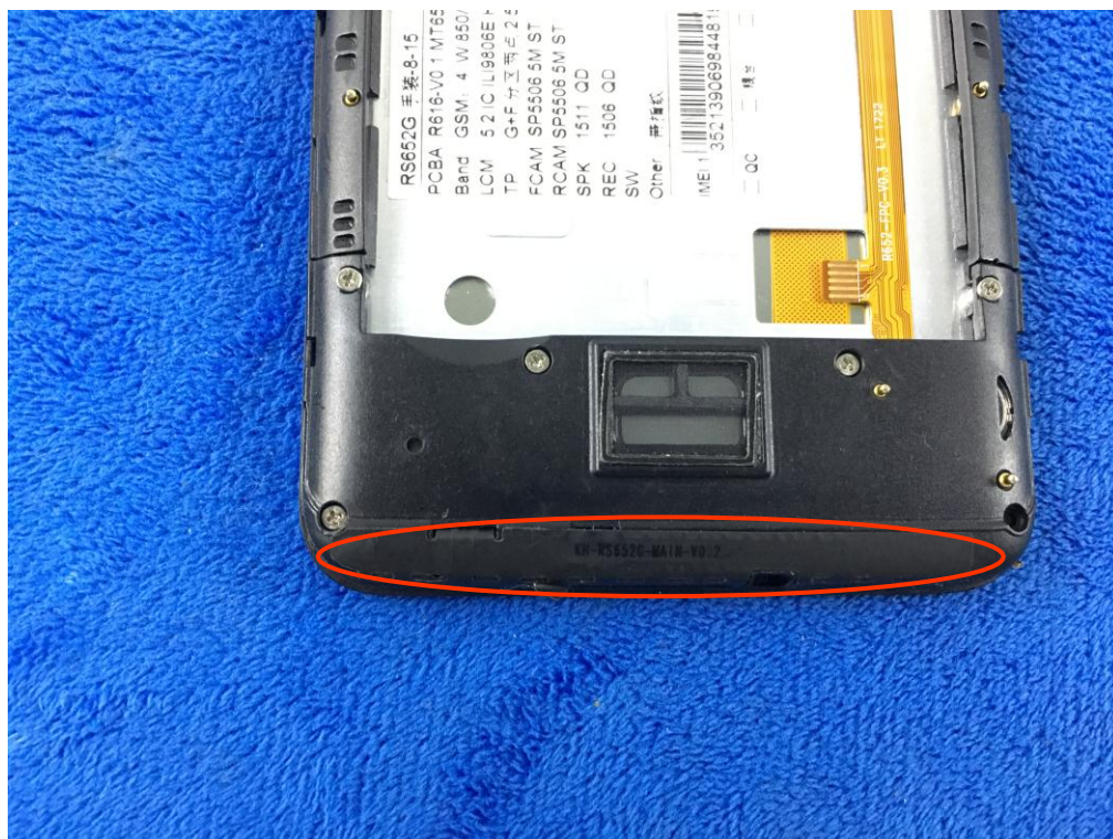
GSM/PCS/UMTS-FDD Antenna View
