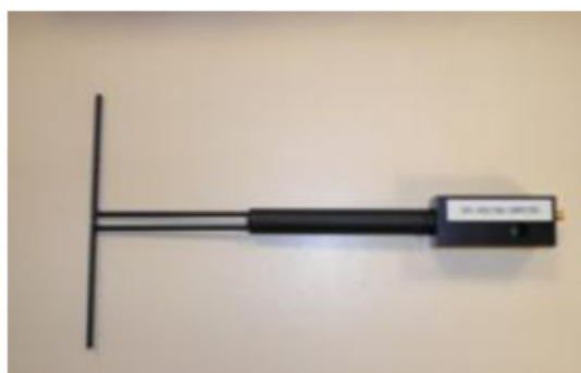
Figure 1 – Satimo COMOSAR Validation Dipole
