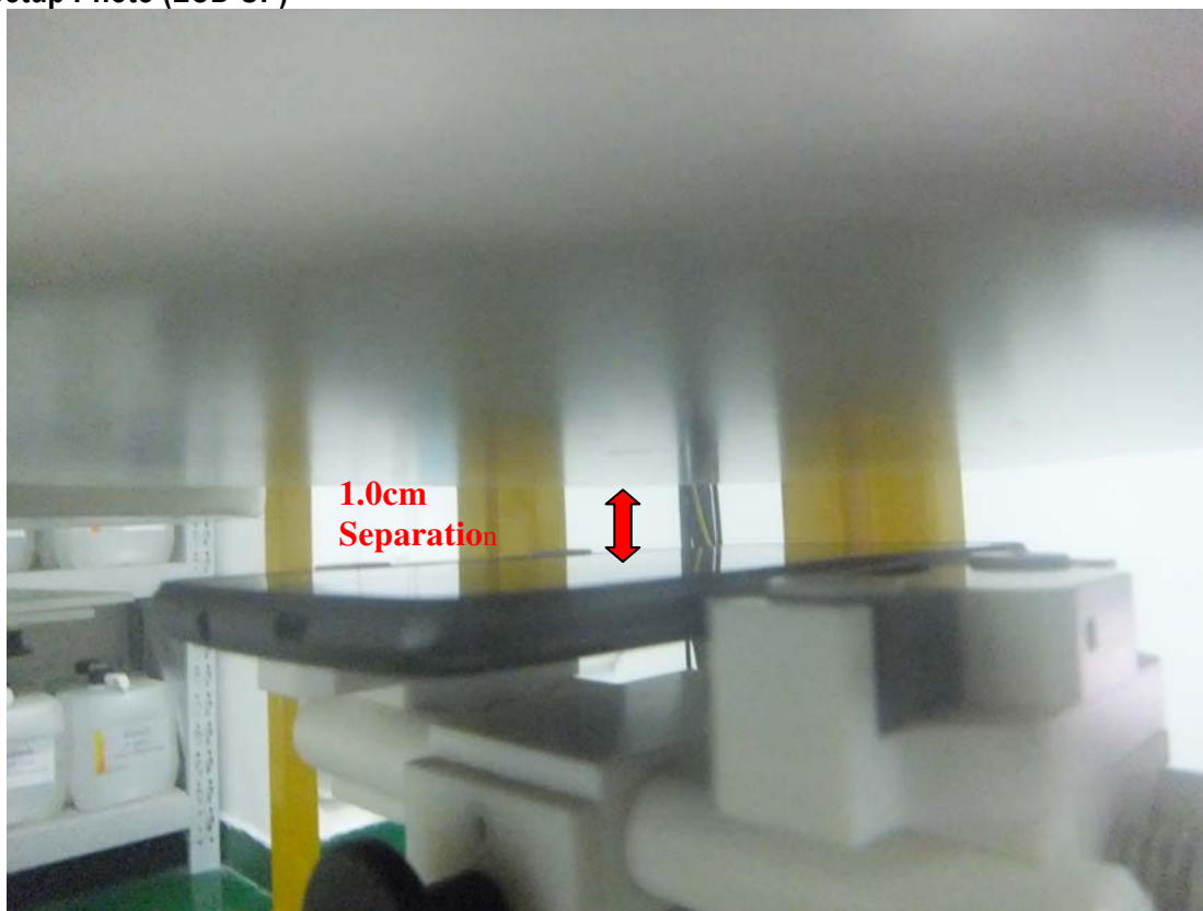
Body Setup Photo (LCD DOWN)
