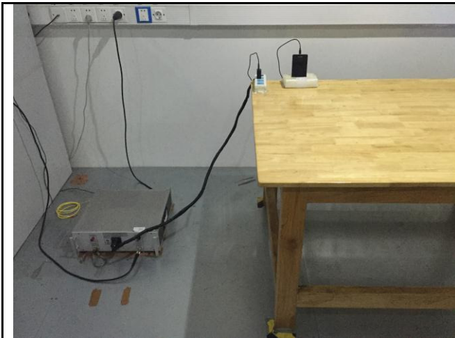
Conducted Emissions Test Setup Front View
