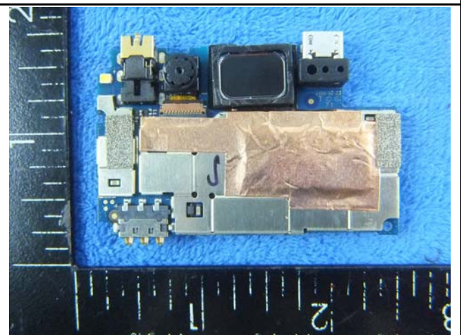
Mainboard with Shielding - Front View
