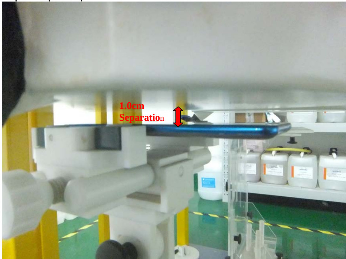
Body Setup Photo (LCD DOWN)
