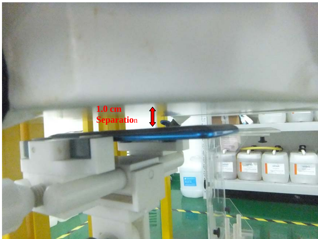
Body Setup Photo (LCD DOWN)
