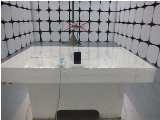
Conducted Emissions Test Setup Front View
