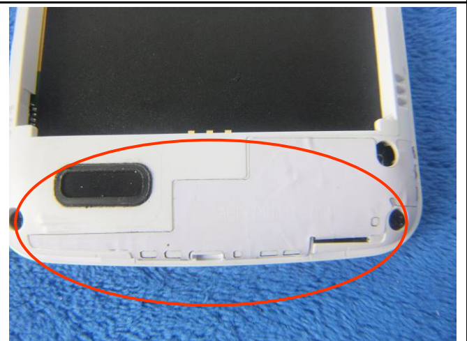
GSM/PCS/UMTS-FDD/LTE - Antenna View
