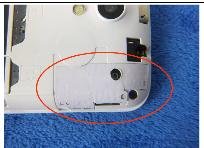
LTE - Antenna View
