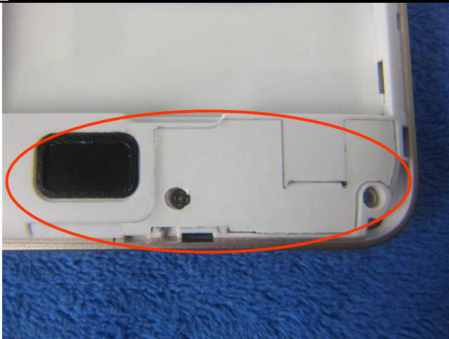
GSM/PCS/UMTS-FDD/LTE Antenna View
