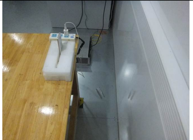
Conducted Emissions Test Setup Side View
