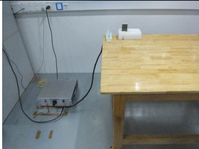
Conducted Emissions Test Setup Front View
