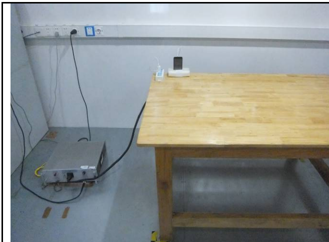
Conducted Emissions Test Setup Front View
