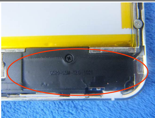
GSM/PCS/UMTS-FDD/LTE Antenna View
