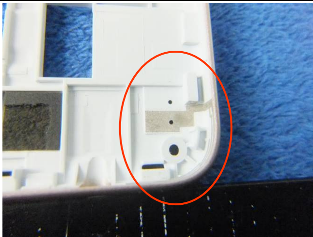
LTE - Antenna View
