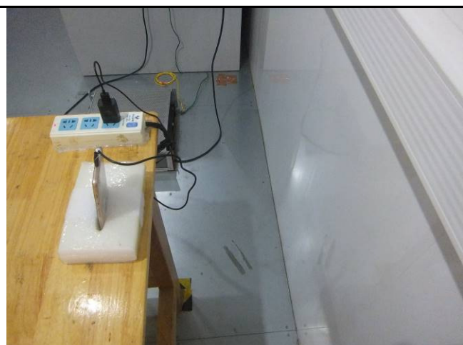
Conducted Emissions Test Setup Side View
