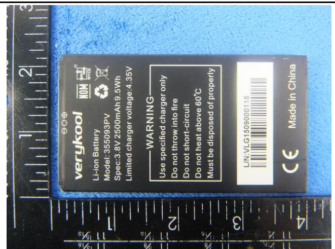
Battery - Rear View
