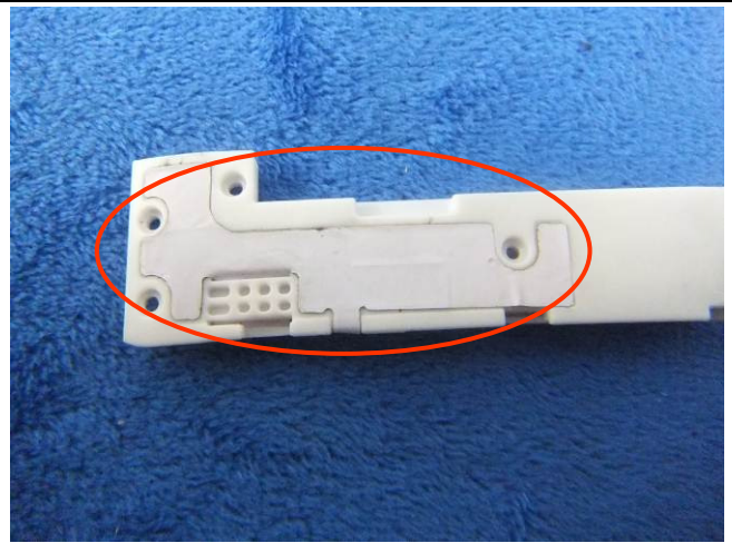
GSM/PCS/UMTS-FDD/LTE Antenna View
