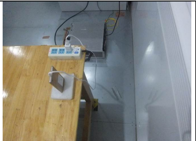
Conducted Emissions Test Setup Side View
