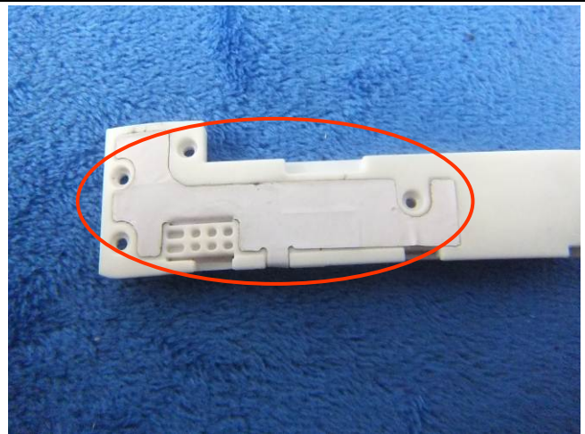
GSM/PCS/UMTS-FDD/LTE Antenna View
