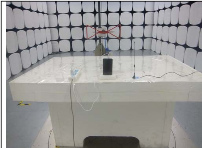
Radiated Spurious Emissions Test Setup Below 1GHz
