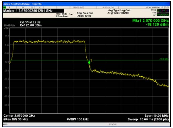
LTE Band 7 - High Channel QPSK-5
