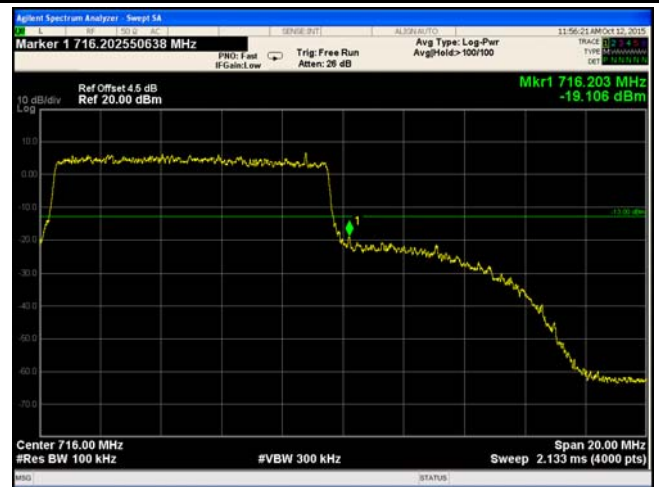
LTE Band 12 - High Channel QPSK-10
