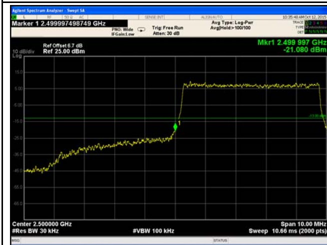
LTE Band 7 - Low Channel 16QAM-5
