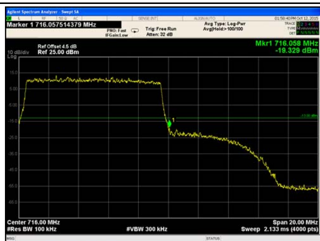
LTE Band 17 - High Channel 16QAM-10
