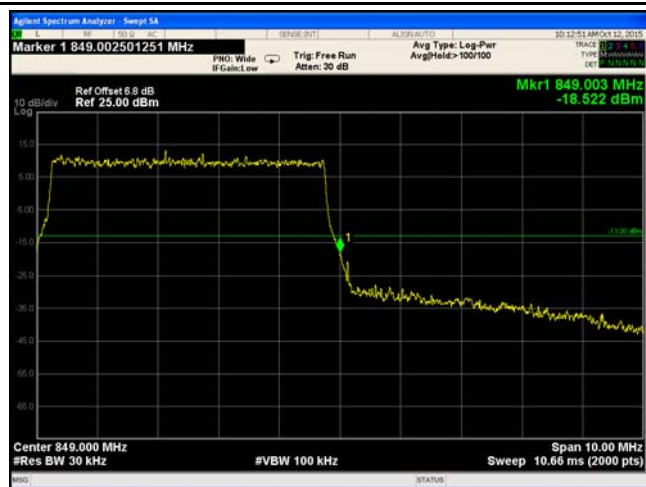
LTE Band 5 - High Channel 16QAM-5
