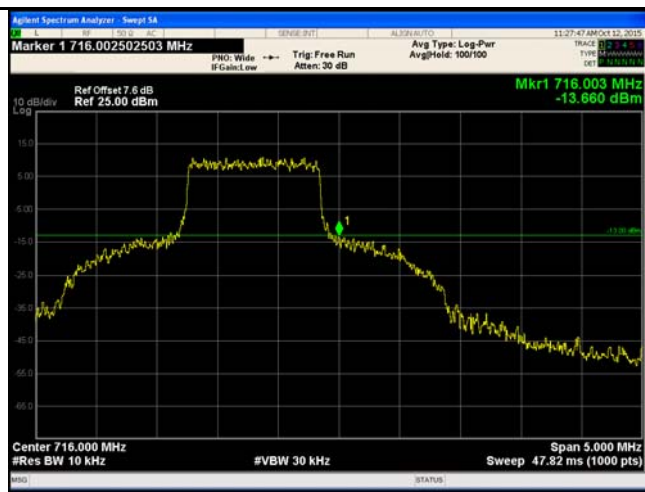
LTE Band 12 - High Channel QPSK-1.4
