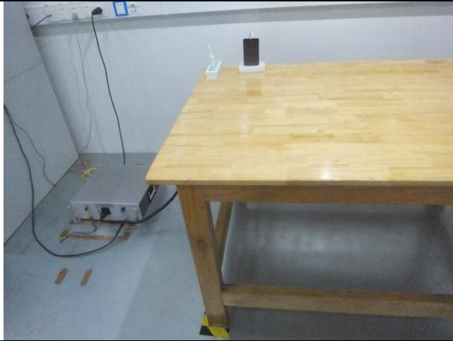
Conducted Emissions Test Setup Front View
