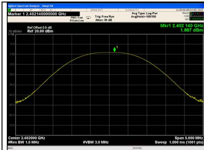
GFSK Output power - Low CH 2402
