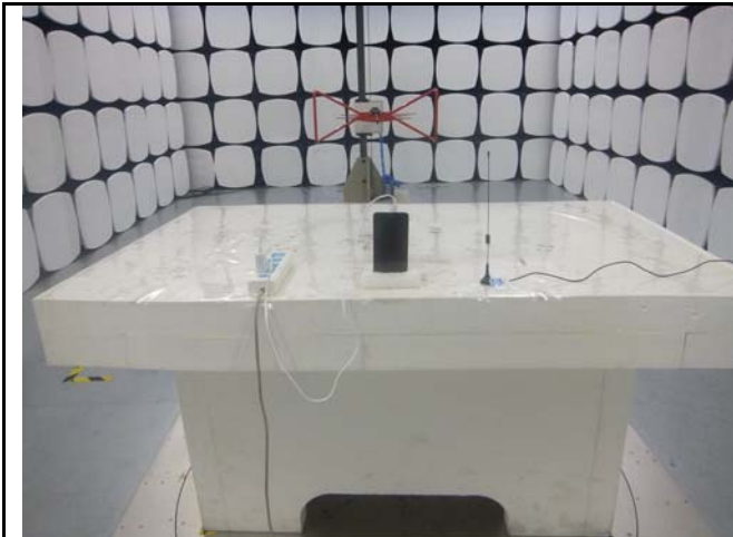
Radiated Spurious Emissions Test Setup Below 1GHz
