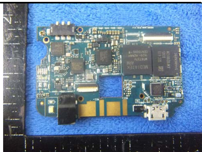
Mainboard without Shielding - Rear View
