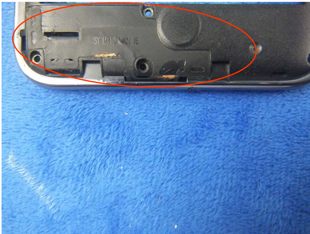
GSM/PCS/UMTS-FDD Antenna View
