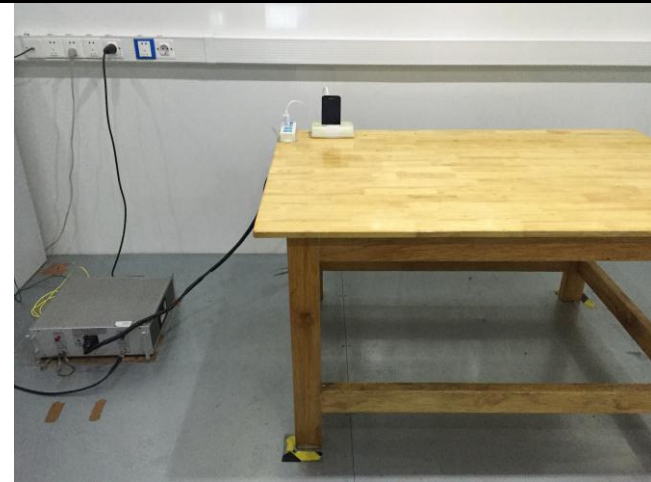
Conducted Emissions Test Setup Front View
