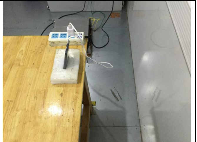
Conducted Emissions Test Setup Side View
