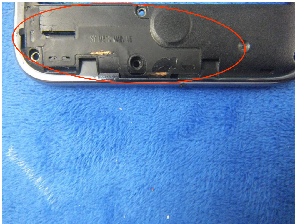
GSM/PCS/UMTS-FDD Antenna View
